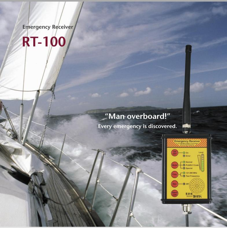
The RT-100 Emergency Receiver monitors the 121.5 MHz international emergency frequency and provides an acoustic alarm if a signal is received on this frequency. At the same time, a relay is activated that can be used to trigger external alarm devices. When the "selective squelch" function is enabled, an alarm is triggered only if the signal is received from an emergency transmitter
